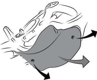
**Remove the original skid plate through the two screws.**
