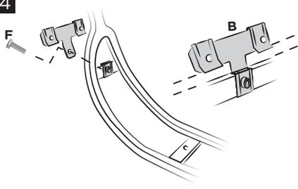
**Assemble the bracket (B) to the original clip on the frame using the original screw (F). Before completely fixing the screw (F), verify that the bracket is parallel to the frame, then fix it.**
