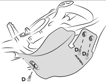
**Place the Acerbis skid plate (A) and check that the holes are aligned with the clips (C). Fix now the Acerbis skidplate (A) with the supplied screws (D).**
