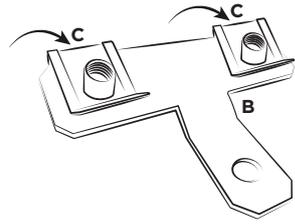
**Assemble the clips (C) on the bracket (B).**
